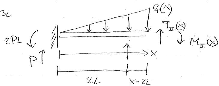
$$T: T_{II}(x) = T_I(x) - P \quad \checkmark: M_{II}(x) = M_I(x) - P(x-2L)$$
