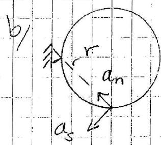
$$a_n = r \omega^2 \quad a_s = r \ddot{\omega} \\ r = \sqrt{2}R \quad \omega = 0 \text{ vid start} \\ a_s = \sqrt{2}R \ddot{\omega} = \text{ins. } a_s = g/\sqrt{2} //$$
