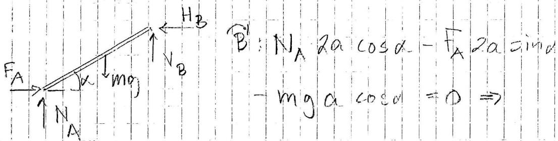
$$\begin{aligned} B: N_A 2a \cos \alpha - F_A 2a \sin \alpha \\ - mg a \cos \alpha = 0 \Rightarrow \end{aligned}$$
