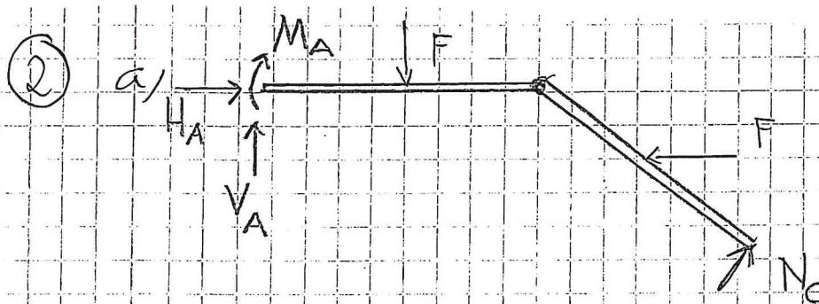
b)  $\rightarrow: H_A - F + N_C / \sqrt{2} = 0 \quad (1) \quad \left. \begin{matrix} H_A = V_A \end{matrix} \right\}$
