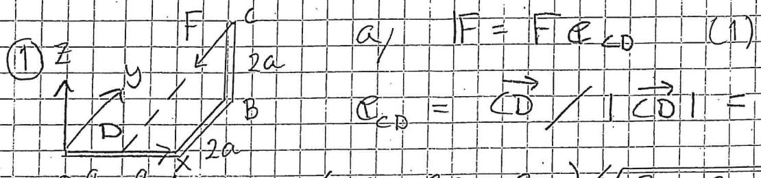
$$e_{CD} = \vec{CD} / |\vec{CD}| = (-a, -2a, -2a) / \sqrt{a^2 + 4a^2 + 4a^2} = \\ = (-1, -2, -2) / 3 // \quad (1) \Rightarrow \bar{F} = F/3 \quad (-1, -2, -2) //$$
