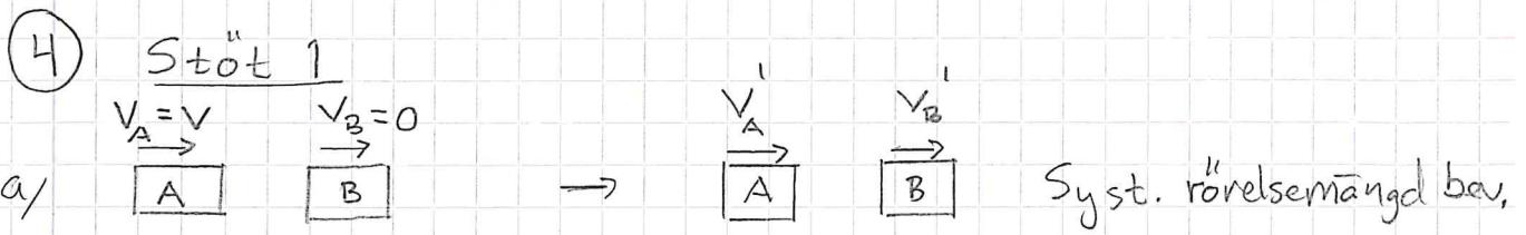
$$\rightarrow : 4mV = 4mV_A' + 2mV_B' ; \quad V_A' = V/2 \Rightarrow V_B' = V \quad (1)$$
