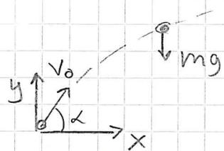
$$\rightarrow: a_x = 0 \Rightarrow V_x = V_0 \cos \alpha \Rightarrow S_x = V_0 t \cos \alpha \quad (1)$$
