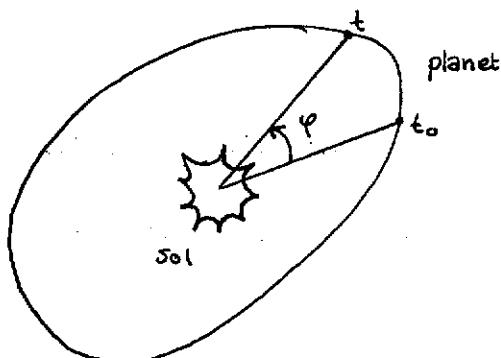
$$\varphi - e \sin \varphi = a(t - t_0)$$
