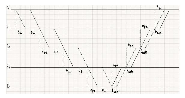
The time required by an Ethernet frame containing the Data-SDU to be transmitted at A, traverse R1, R2, R3, and be received at B can be expressed as:
