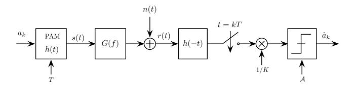
The channel frequency response is defined in the figure below.
