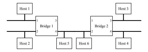
Whenever a bridge receives a frame on one of its ports, the frame will subsequently be forwarded (transmitted) on none, one, or several of the bridge ports. For example, suppose that (i) H1 transmit a frame F, which is received by B1 on its port 1, and (ii) that the bridge forward the frame on its ports 2 and 4, which is received by H2, H5, H6, and B2 on port 2. The transmission-and-reception cycles (i) and (ii) can be described in table format as
