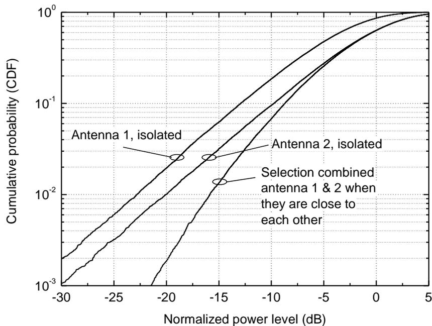
**Figure 3.1. CDF:s for the two dipole antennas measured separately without the other antenna present and when placed close to each other when selection combination is used, respectively.**
