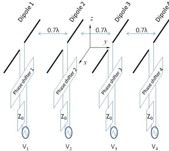
Figure 4.3 A 4-dipole linear array antenna
