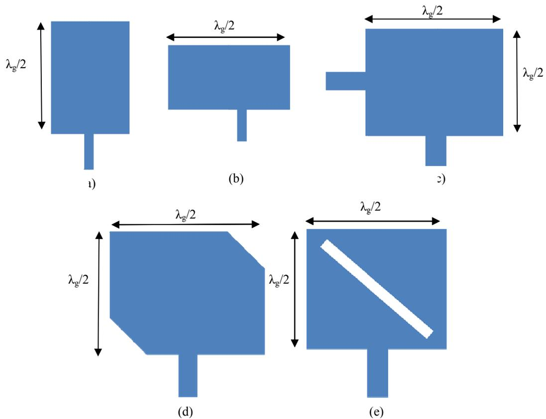
**Figure 1.4 different patch antennas.**
