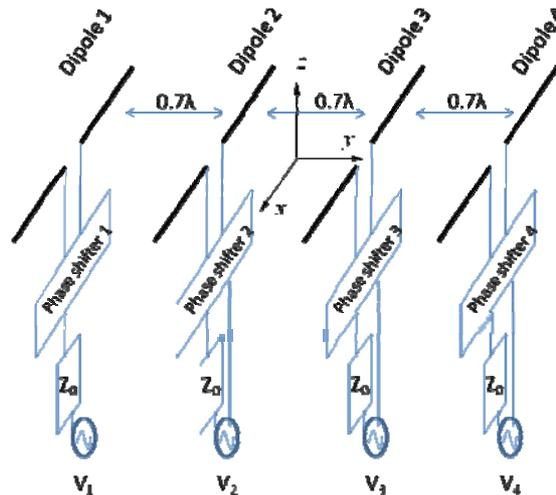
Figure 4.3 A 4-dipole linear array antenna
