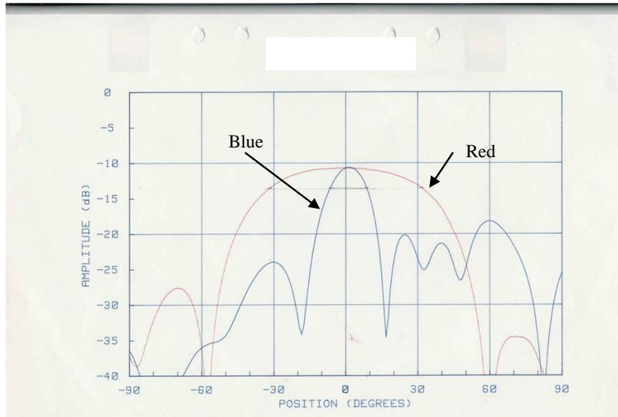
**Figure 1.2 Measured radiation patterns on both E- and H-planes for antenna 1**
