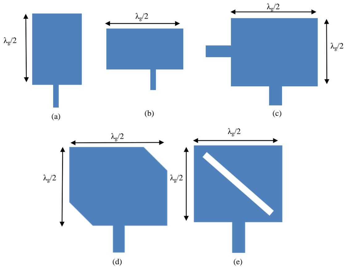
**Figure 1.4 different patch antennas.**
