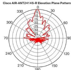
(c) Cisco AIR-ANT2414S-R Elevation Plane Pattern
