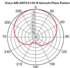
(b) Cisco AIR-ANT2414S-R Azimuth Plane Pattern
