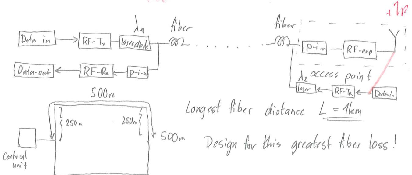
The frequency used for the design is  $f = 900$  MHz (downlink) (for mobile phone users)
