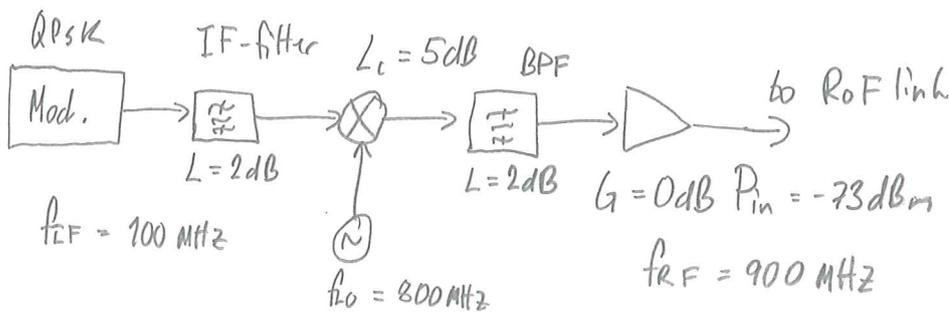
IF-filter  $\left\{ \begin{array}{l} f_c = 100 \text{ MHz} \\ \Delta f = 5 \text{ MHz} \end{array} \right. \Rightarrow \frac{\Delta f}{f} = 5\% \text{ OK!}$
