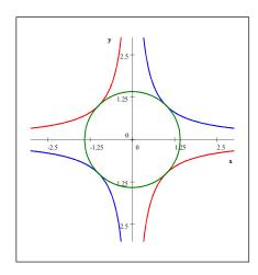
All trajectories starting in this circle stay in it and must have an  $\omega$  limit set there.  $V_f^{-1}(0)$  consists of only the origin. According to the LaSalles invariance principle all solutions starting inside the circle  $x^2 + y^2 < 2$  must tend to the origin, that is an asymptotically stable equilibrium point. Therefore the domain  $x^2 + y^2 < 2$  is the domain of attraction for the equilibrium point in the origin.
