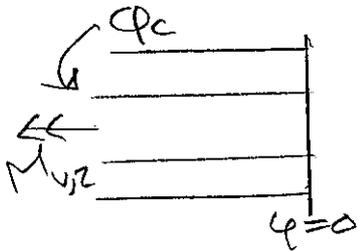
$$\begin{aligned} \phi_c &= \frac{-M_{y2} \cdot 3L}{G K_{\text{③}}} = \left\{ K_{\text{③}} = \frac{\pi}{2} \left( \left( \frac{D}{2} \right)^4 - \left( \frac{d}{2} \right)^4 \right) \right\} = \\ &= \frac{-7776}{65} \cdot \frac{M_{y2} L}{\pi G D^4} \end{aligned}$$
