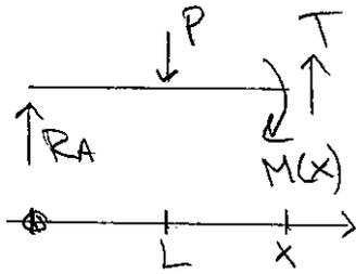
$$\begin{aligned} M(x) &= -R_A x + P(x-L) \\ &= P(x-L) + \frac{R_B x}{2} - \frac{3Px}{4} \end{aligned}$$
