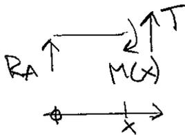
$$\frac{\partial M}{\partial P} = -\frac{x}{2}, \quad \frac{\partial M}{\partial M_0} = -\frac{x}{2L}$$
