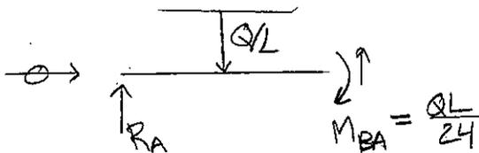
$$\curvearrowright B: R_A \cdot L - \frac{Q}{L} \cdot L \cdot \frac{L}{2} + \frac{QL}{24} = 0, \quad R_A = \underline{\underline{\frac{11Q}{24}}}$$
