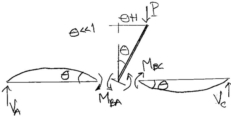
$$\text{F.s. stiel } q: \left. \begin{aligned} \theta &= \frac{M_{BA} L}{3EI} \\ \theta &= \frac{M_{BC} L}{3EI} \end{aligned} \right\} \Rightarrow M_{BA} = M_{BC} = \frac{3EI}{L} \cdot \theta$$
