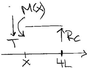
$$\begin{aligned} M(x) &= \frac{R_B}{2}(4L-x) - \frac{P}{4}(4L-x) \\ &\quad (-R_C(4L-x)) \end{aligned}$$
