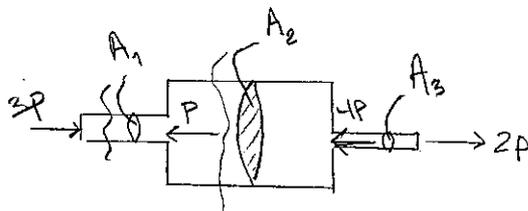
$$\begin{aligned} A_1 &= 75 \text{ mm}^2 \\ A_2 &= 100 \text{ mm}^2 \\ A_3 &= 50 \text{ mm}^2 \\ P &= 2 \text{ kN} \end{aligned}$$
