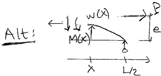
$$\begin{aligned} \leftarrow x \right) : M(x) - P(e - w(x)) &= 0 \\ M(x) &= Pe \left( 1 - 1 + \frac{\cosh(nx)}{\cosh\left(\frac{nL}{2}\right)} \right) \end{aligned}$$
