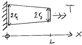
$$r(x) = r_1 - \frac{x}{L}(r_1 - r_2)$$
