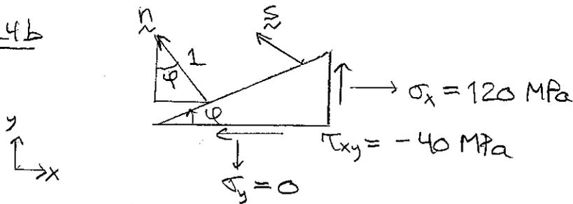
$$\sigma_z = -100 \text{ MPa}, \tau_{yz} = \tau_{xz} = 0, \varphi = 30^\circ$$
