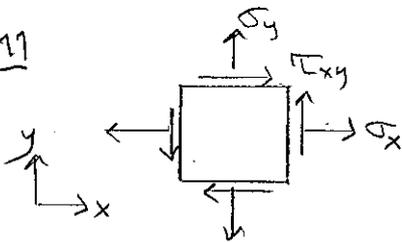
$$\begin{aligned} \sigma_x &= 120 \text{ MPa}, \quad \sigma_y = 70 \text{ MPa} \\ \tau_{xy} &= 60 \text{ MPa} \end{aligned}$$
