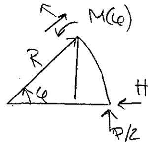
$$\curvearrowleft : M(\varphi) - HR \sin \varphi + \frac{PR}{2} (1 - \cos \varphi) = 0$$
