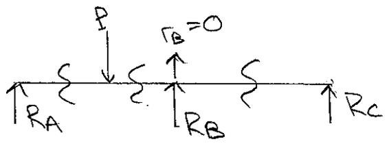
$$\curvearrow C : R_A \cdot 4L - P \cdot 3L + R_B \cdot 2L = 0, \quad R_A = \frac{3P}{4} - \frac{R_B}{2}$$
