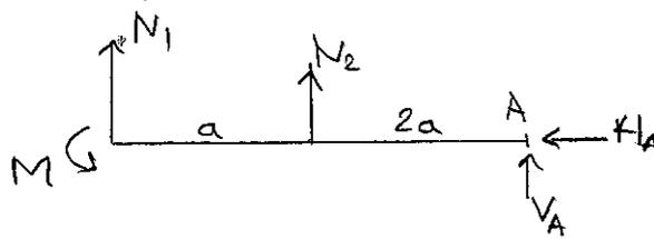
$$\begin{aligned} \curvearrowleft A: N_1 \cdot 3a + N_2 \cdot 2a - M &= 0 \\ 3N_1 + 2N_2 &= \frac{M}{a} \quad (1) \end{aligned}$$
