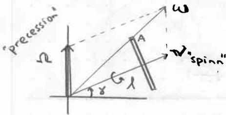
Givet:  $\gamma = 30^\circ$ ,  $r = 0.125 \text{ m}$ ,  $l = 0.25 \text{ m}$
