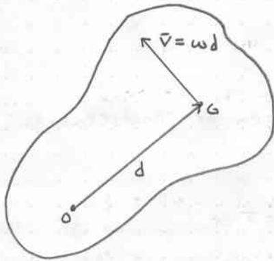
$$T = \begin{cases} \frac{1}{2} m \bar{v}^2 + \frac{1}{2} \bar{I} \omega^2 = \frac{1}{2} (I + m d^2) \omega^2 \\ \frac{1}{2} I_0 \omega^2 \end{cases}$$
