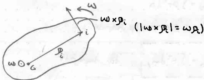
$$L_G = \sum_i p_i \times p_i = \sum_i p_i \times m_i (\omega \times p_i)$$
