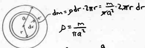
$$\bar{I} = \int_0^a r^2 dm = \int_0^a \frac{m}{a^2} \cdot 2\pi r^3 dr = \frac{2m}{a^2} \left[ \frac{1}{4} r^4 \right]_0^a = \frac{m a^2}{2}$$
