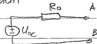
$$U_{oc} = -18 \text{ V}, \quad R_0 = 3 \text{ k}\Omega$$
