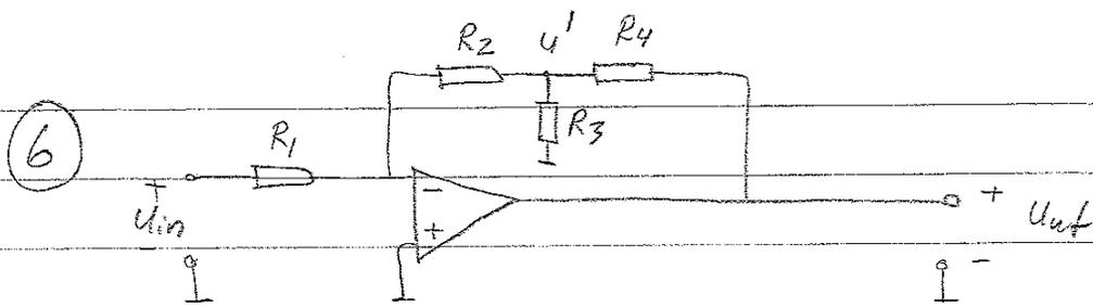
$$\left. \begin{aligned} \frac{U_{in}}{R_1} + \frac{U'}{R_2} &= 0 \Rightarrow U' = -\frac{R_2}{R_1} U_{in} \\ \frac{U_{in}}{R_1} + \frac{U_{out} - U'}{R_4} &= \frac{U'}{R_3} \end{aligned} \right\} \begin{array}{l} \text{Ideal op-amp} \\ \text{Neg. o'tok} \\ \Rightarrow \varepsilon = 0 \end{array}$$
