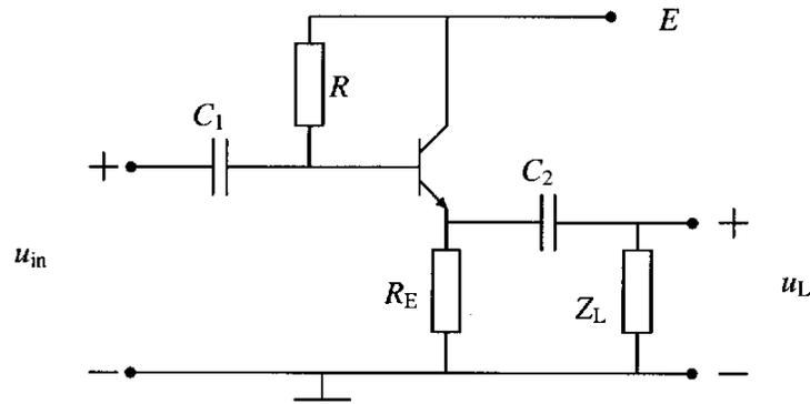
$$R = 500\ \text{k}\Omega, R_E = 5\ \text{k}\Omega, E = 12\ \text{V}$$
