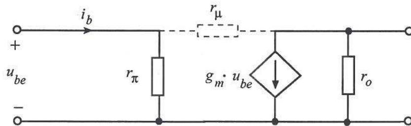
$$g_m = \frac{|I_C|}{V_T} \quad h_{ie} = r_\pi \quad \left( r_\mu = \frac{r_\pi}{h_{re}} \right)$$
