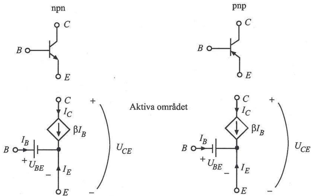
$$\begin{aligned} I_B &> 0 \\ U_{CE} &> U_{CE_{sat}} \\ U_{BE} &\approx E_0 \\ \beta I_B &= I_C \end{aligned}$$
