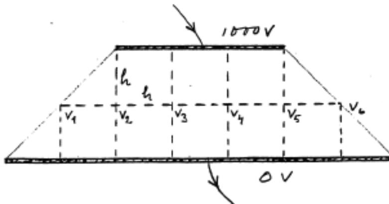
② A)  $R_{\text{ö}} = \frac{1}{\sigma d} \cdot \frac{2h}{3h} = \frac{1}{\sigma d} \cdot 0.6667$  (Lodrieta strömlinjer)
